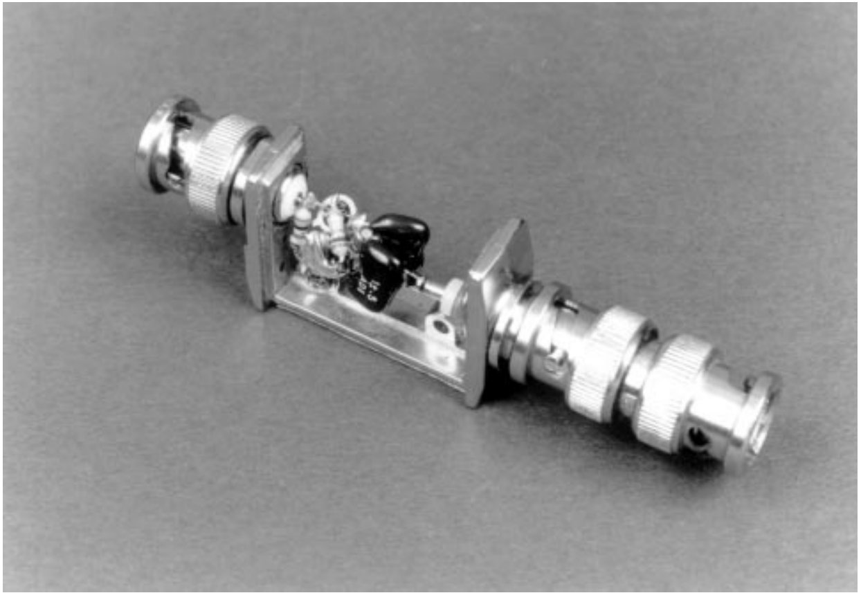
Figure B3. Details of the Avalanche Pulse Generator's Head. 90VDC Enters at Lower Right BNC, Pulse Exits at Top Left BNC. Note Short Lead Lengths Associated with Output
